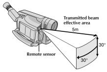
When using the remote control, be sure to point it at the remote sensor. The illustration shows the approximate transmitted beam effective area for indoor use.
